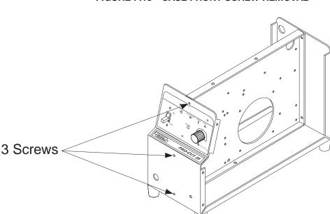
FIGURE F.15 - CASE FRONT SCREW REMOVAL
